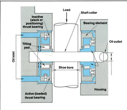
Tilting-pad thrust bearings normally are used in pairs. One bearing carries the load; the other positions the shaft and carries transient reverse thrust loads. A slight pressure inside the bearing housing effectively discharges the oil to minimize churning losses.
