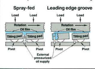
would have a negative impact on bearing capacity. The tendency of the small orifices to clog has the potential to further reduce oil supply flow rate, which could deprive the bearing of the oil necessary to form a full hydrodynamic wedge, creating a situation that can lead to bearing failure.
